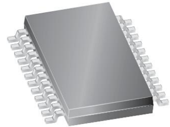
24 pin TSSOP with exposed thermal pad
